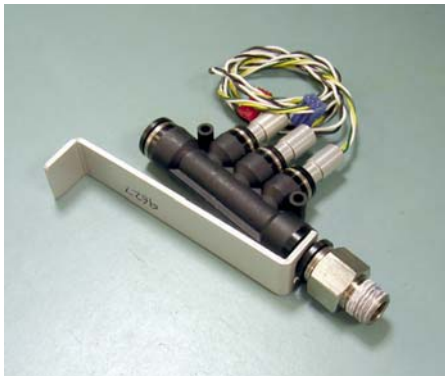
Pisco Fitting Removal Tool (Fitting is inside BAM)
