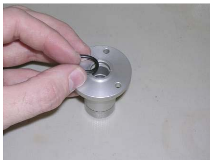
Replacing the nozzle o-ring
